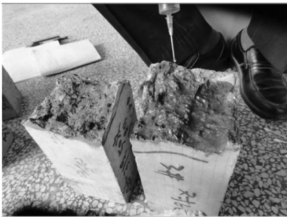
图 4 铬酸钾变干后滴加硝酸银 Fig. 4 Add silver nitrate after potassium chromate dry
