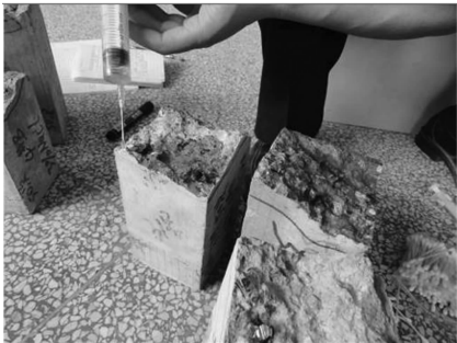
图 3 试件断面上滴加铬酸钾 Fig. 3 Add potassium chromate on the sections
