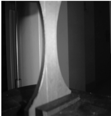
图 2 试样拉伸断裂前瞬间图 Fig.2 The specimen was stretched to fracture
