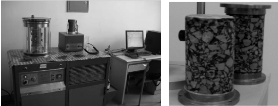
图 1 SPT 试验设备及试件 Fig.1 SPT equipment and samples
