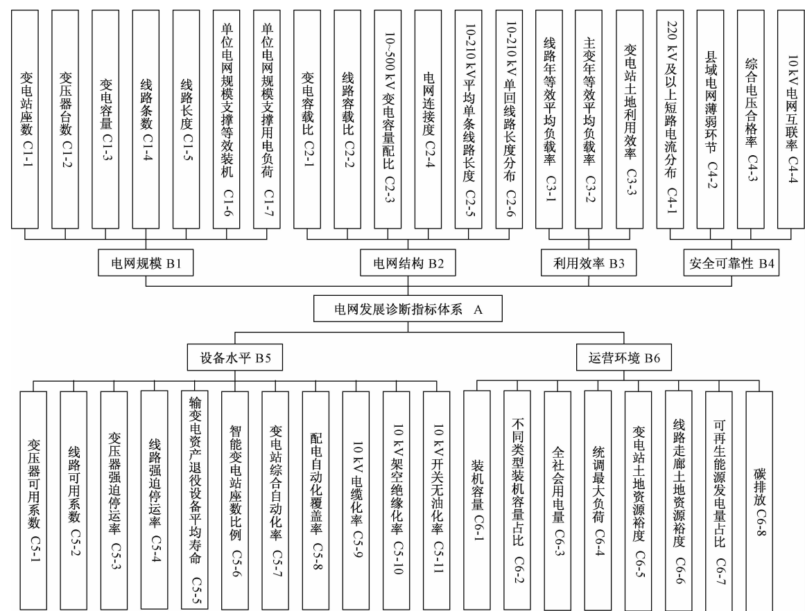
图 1 电网发展诊断指标体系 Fig.1 The index system of power grid development diagnosis
