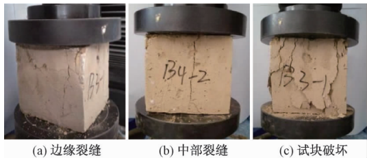
图 3 掺合稻草粗砂试块抗压强度试验破坏过程 Fig.3 Failure process specimens with rice straw and rough sand during compressive strength tests
