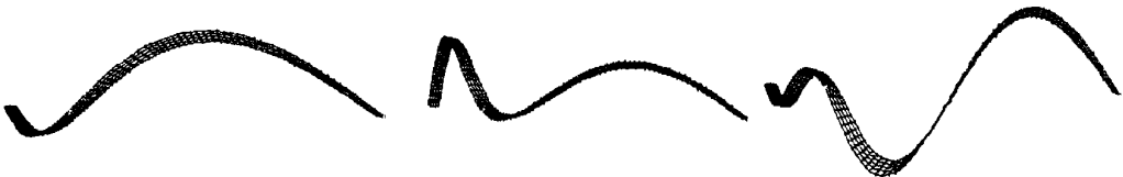
图 8 竖向前三阶振型示意 Fig .8 The former three modal shapes in the vertical direction
