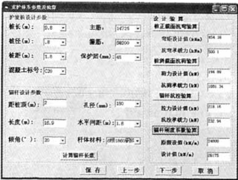
图 7 支护结构设计参数及验算 Fig.7 Design parameters of a retaining structure and checking computations
