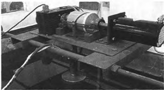
图 1 窄带超声探测装置 Fig.1 Narrowband echo exploration system
