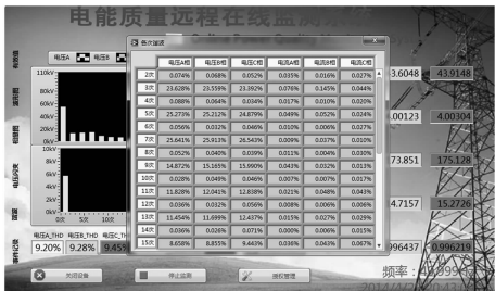
图 5 实时谐波分析与频谱 Fig.5 Real-time harmonic analysis and frequency spectrum
