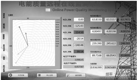
图 6 三相不平衡实时分析 Fig.6 Real-time analysis of three phase imbalance
