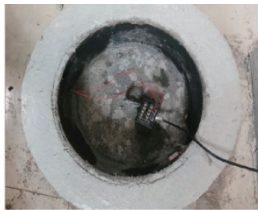
图 3 桥面混凝土约束收缩试验 Figure 3 Confined shrinkage test of bridge deck concrete
