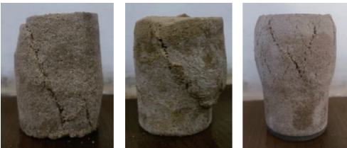
(a) 整体剪坏破坏 (b) 局部剪切破坏 (c) 鼓胀剪切破坏
