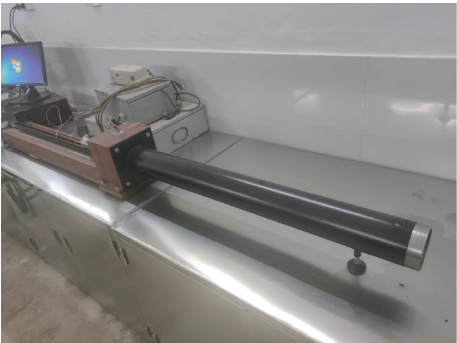
图 1 AWA6128A 型驻波管 Figure 1 AWA6128A standing wave tube
